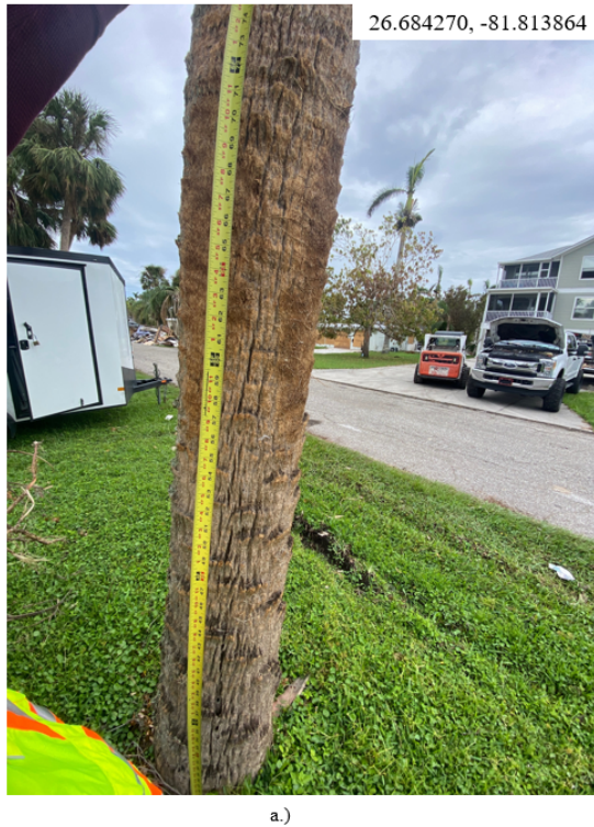
Figure 4.22: Evidence of the storm surge in Cape Coral: (a) debris marks on trees measuring at 72 inches (b) closer look at the debris marks
