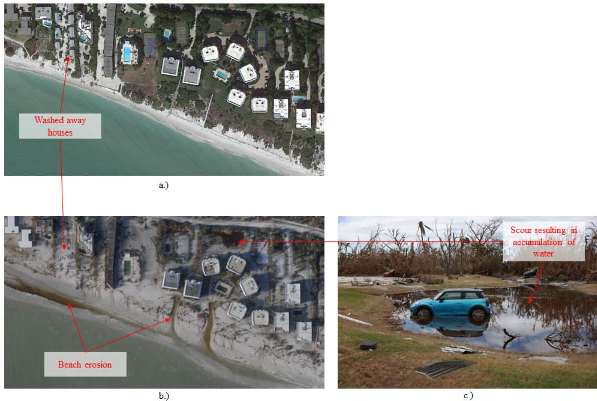
Figure 4.56: Effects of Hurricane Ian on Sanibel Island's shoreline: (a) pre-hurricane satellite photo; (b) post-hurricane satellite photo showing extreme beach erosion more pronounced on the path of the walkways; (c) ground depression and accumulation of water. Coordinates: 26.42657, -82.10010
