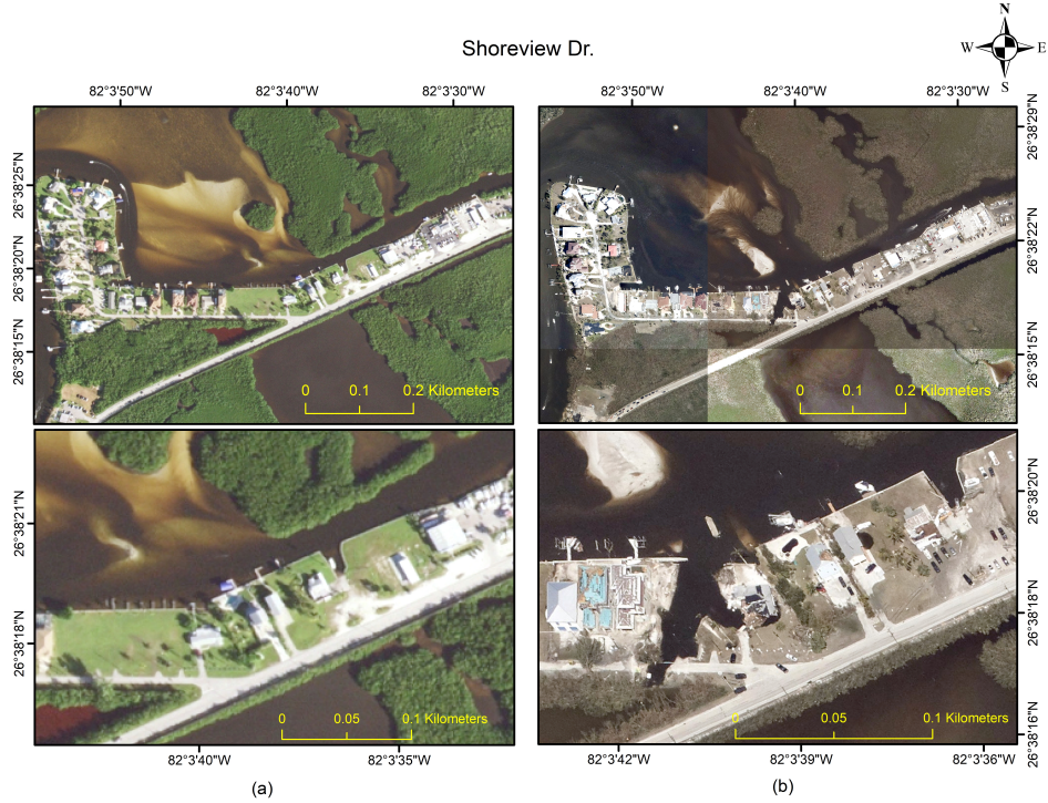
Figure 4.2: Satellite photos of Shoreview Drive in Matlacha Isles-Matlacha Shores at different scales (top vs. bottom) a.)before and b.)after Hurricane Ian, where it can be seen that a section of the sea wall and Shoreview Drive were eroded away and made impassable immediately after the storm. Note that the home shown immediately west of the eroded region was under construction and is not shown pre-event satellite imagery.
