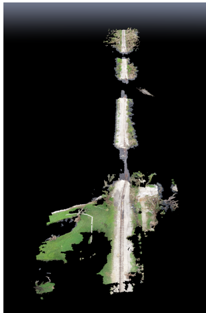
Figure 4.50: Structure from Motion photogrammetry model of rail bridge failure across the Caloosahatchee River. Coordinates: 26.6922922, -81.8123293
